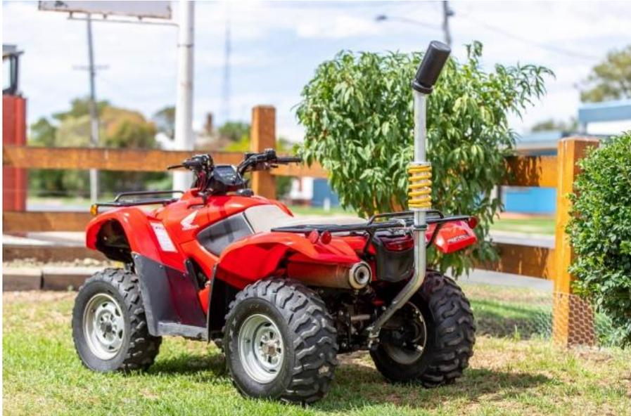
1) Full-scale tests on the use of ROPS on Quadbikes
